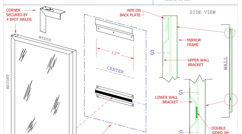
ONE PIECE 18 GA. 5/8 X 5/8 TYPE. 304 SATIN STAINLESS STEEL FRAME WITH TIGHTLY MITERED CORNERS.
